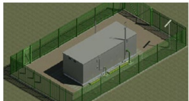
Figure 3-36: Biomethane Network Entry Facility (Prefabricated Unit - Illustration) (Gas Networks Ireland)
