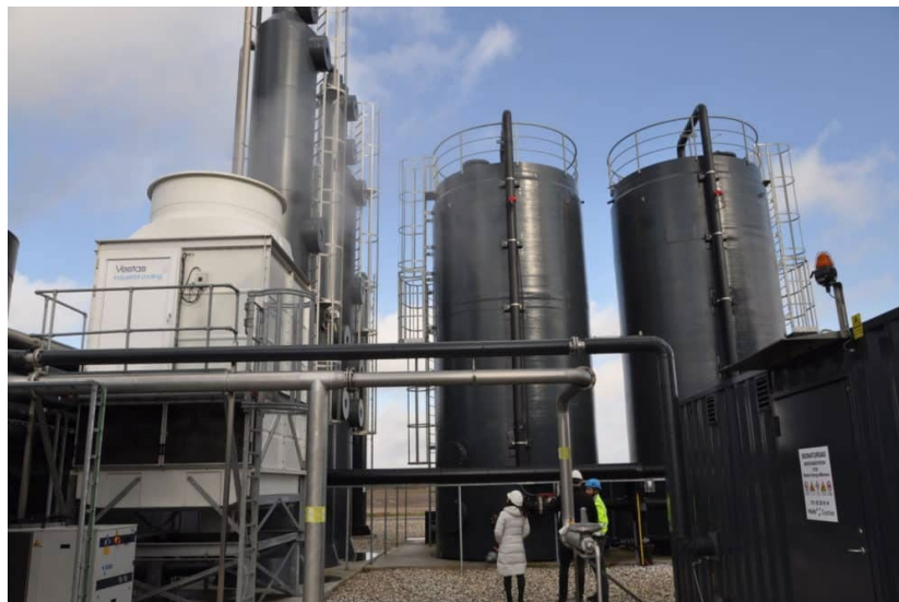
Figure 3-34: Amine Biogas Upgrader – Ammongas (World Biogas Association, 2026)
